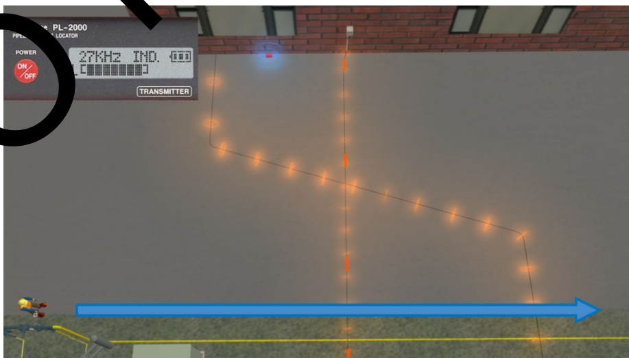
2-36 Parallel Line Check (transmitter left of known line) – Crossing Line Detected
