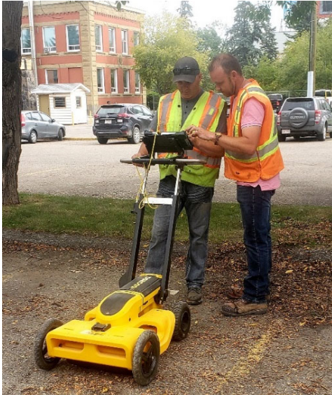
4-19 Using GPR in an urban environment
